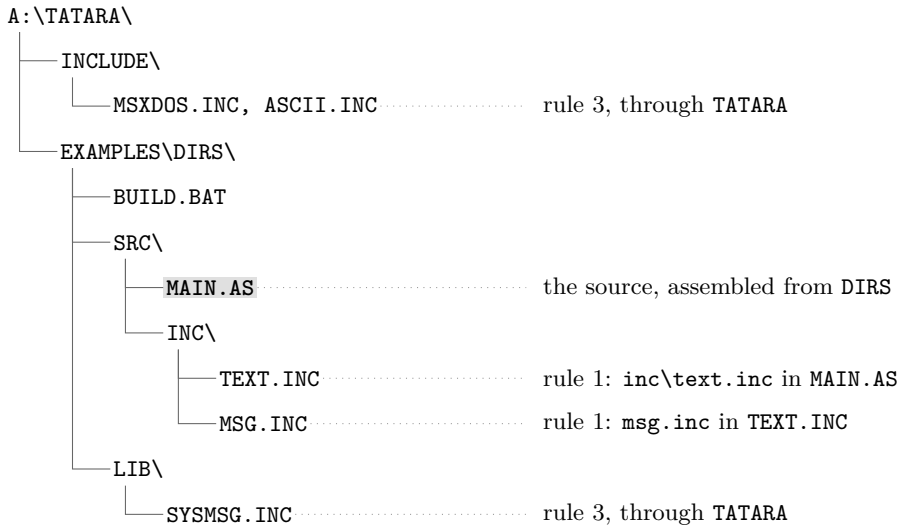
Figure 34.1: The files of DIRS, and the rule that finds each include file.
